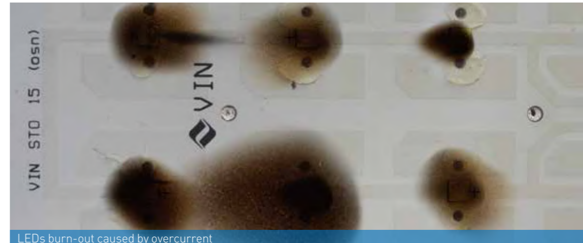
LEDs burn-out caused by overcurrent
